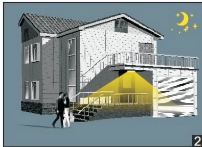
With insufficient daylight,even when motion detected.light ON.
